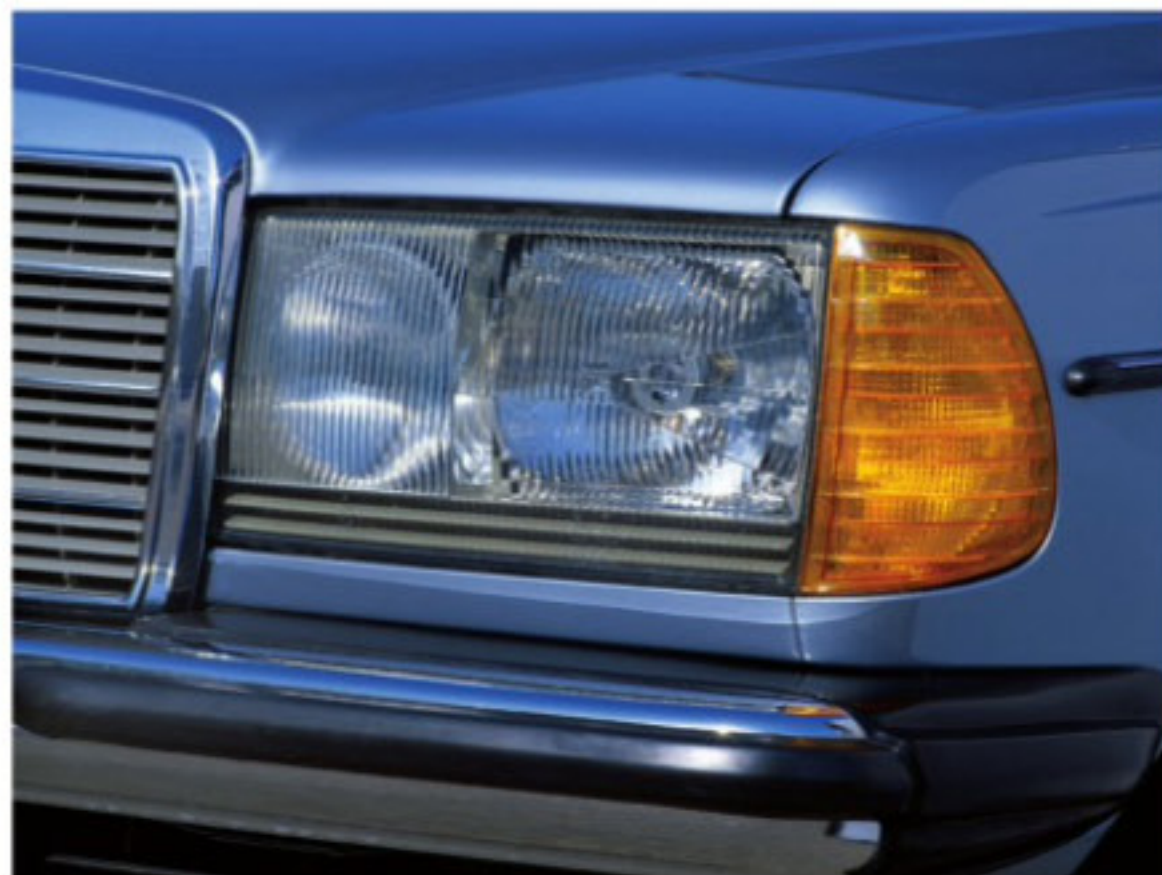
ABOVE Headlights and driving lamps were positioned behind a single glass lens.
