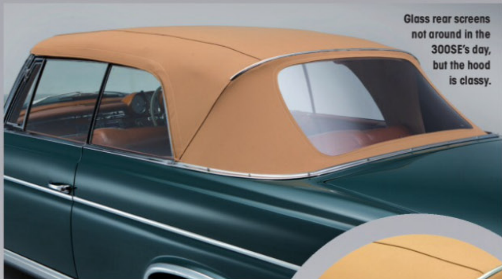
A gap free join with the screen and side window minimises wind noise.
