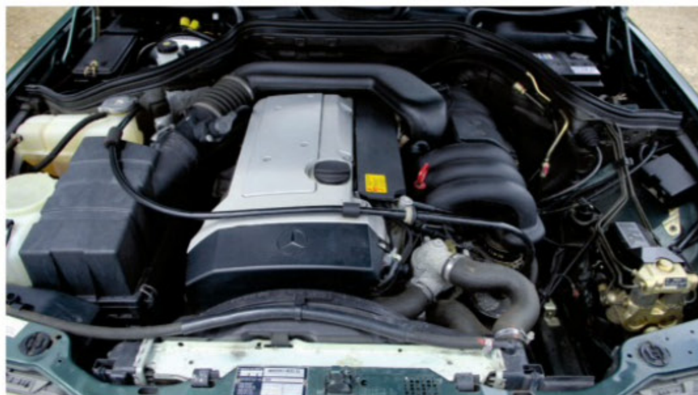
BELOW Sweet M104, 24-valve 3.2-litre was Mercedes’ final petrol straight-six.
